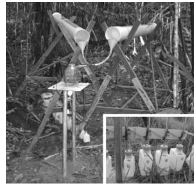
Fig. 1 Sequential sampler design: Composite of two through collectors, a tipping bucket and 10 sampling bottles. The detail image in the lower right image corner shows individual sampling bottles and the connection tubing
